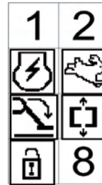
Fig. 141 Emergency BY-PASS activated
