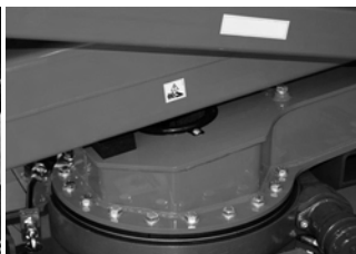
Fig. 107 Example potential shearing risk zone 2
