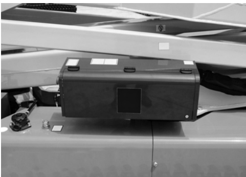
Fig. 134 Aerial part distributor protection
