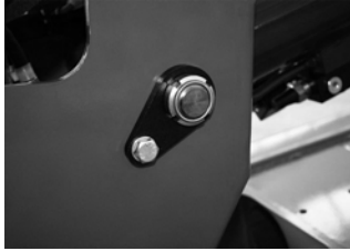
Fig. 28 Bolts to stop rotation
