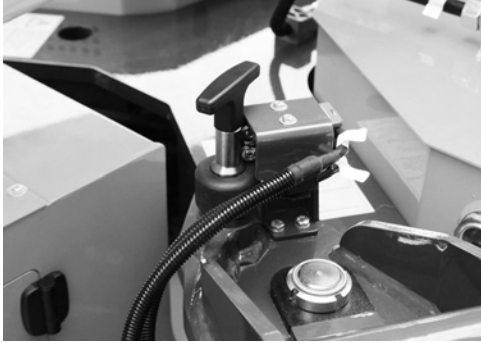
Fig. 94 Check outrigger lock
