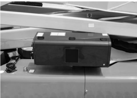
Fig. 122 Aerial part distributor protection
