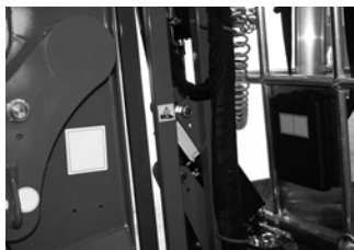
Fig. 106 Example potential shearing risk zone 1
