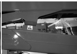
Fig. 108 Example potential shearing risk zone 3
